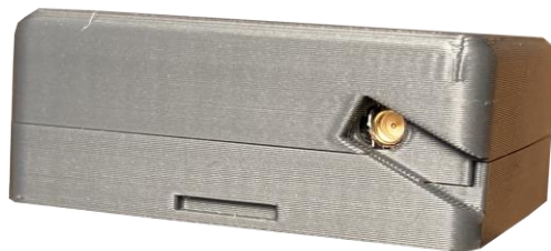
Figure 1 ADL165 Back side with MMCX Iridium antenna connector
