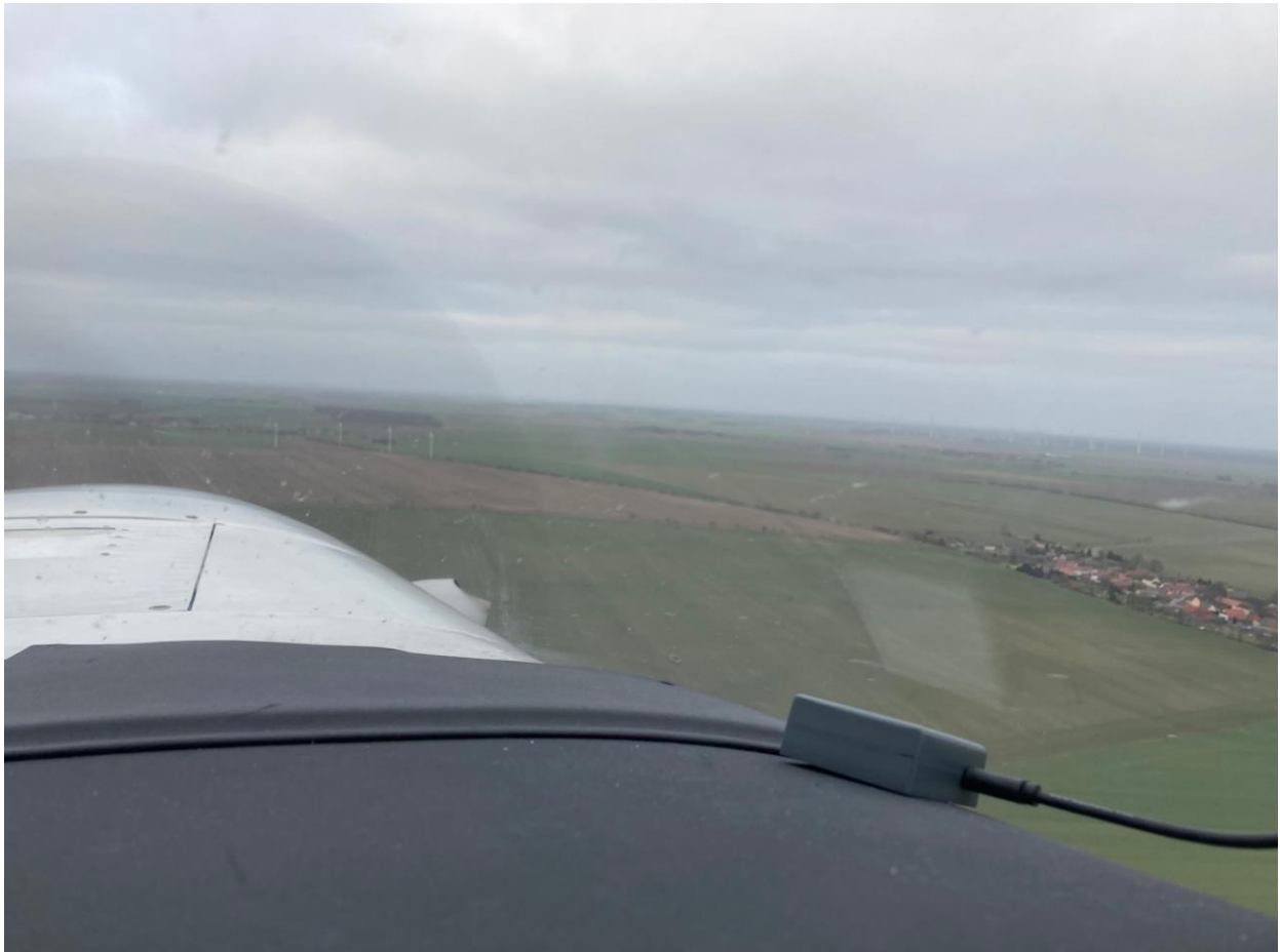
Figure 3 ADL165 on the glare shield in the right orientation
