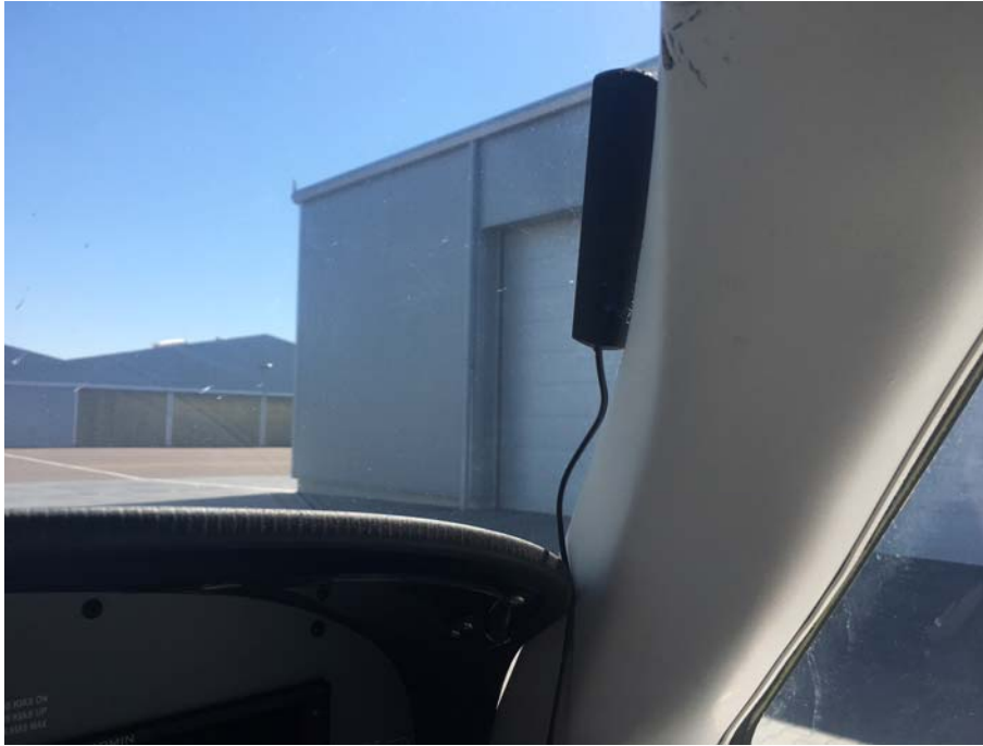
Figure 10 ADS-B Antenna Example
