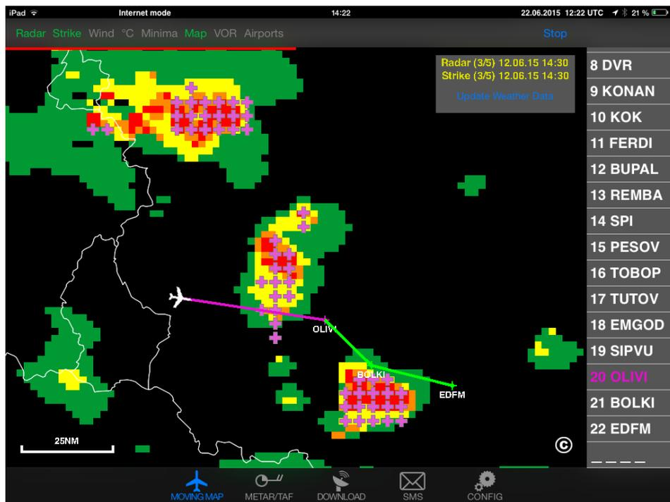
Combining the radar with the strike images helps to verify that radar system is working properly. Strike data is processed separately except for the final display. So if the strikes line up with the radar data this is a good indication the whole system is working properly.
