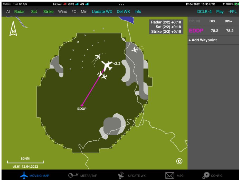
Figure 8 ADLConnect Showing the Latest Weather Data and Traffic from ADL200
